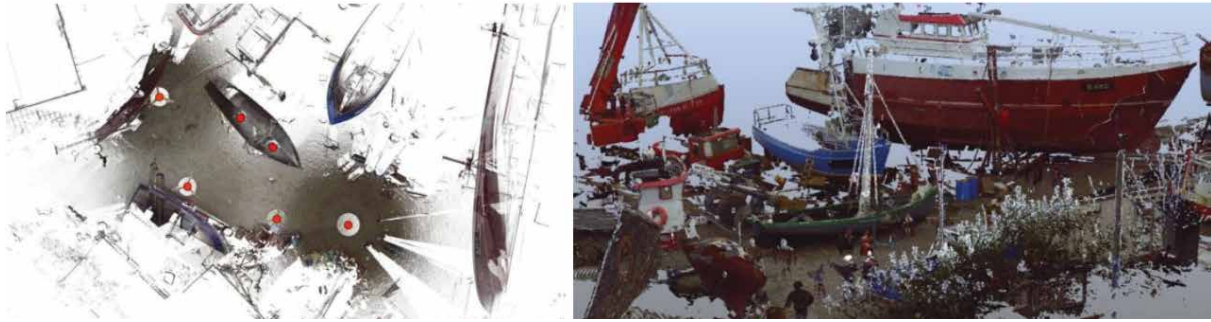
Fig. 3 3D laser scanning a 9 m vessel (author: Pat Tanner)
