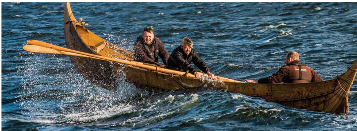
Fig. 3 Rowing tests conducted in 2015 on Roskilde Fjord with Gisle, one of the Viking Ship Museum's Gislinge Boat reconstructions. The Gislinge Boat is a boat-find from Zealand, Denmark dated to ca. 1130 (photo: W. Karrasch, Viking Ship Museum in Roskilde).
