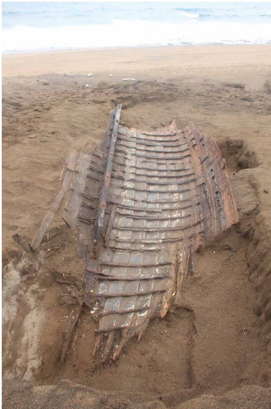
Fig. 6 View of the Gorrondatxe boat fully excavated, with the sea washing over the beach. This is the second modern clinker-built boat found, dated to the late 19 th or early 20 th century and abandoned or wrecked in the 1960s or 1970s (photo: J. M. Matés Luque).
