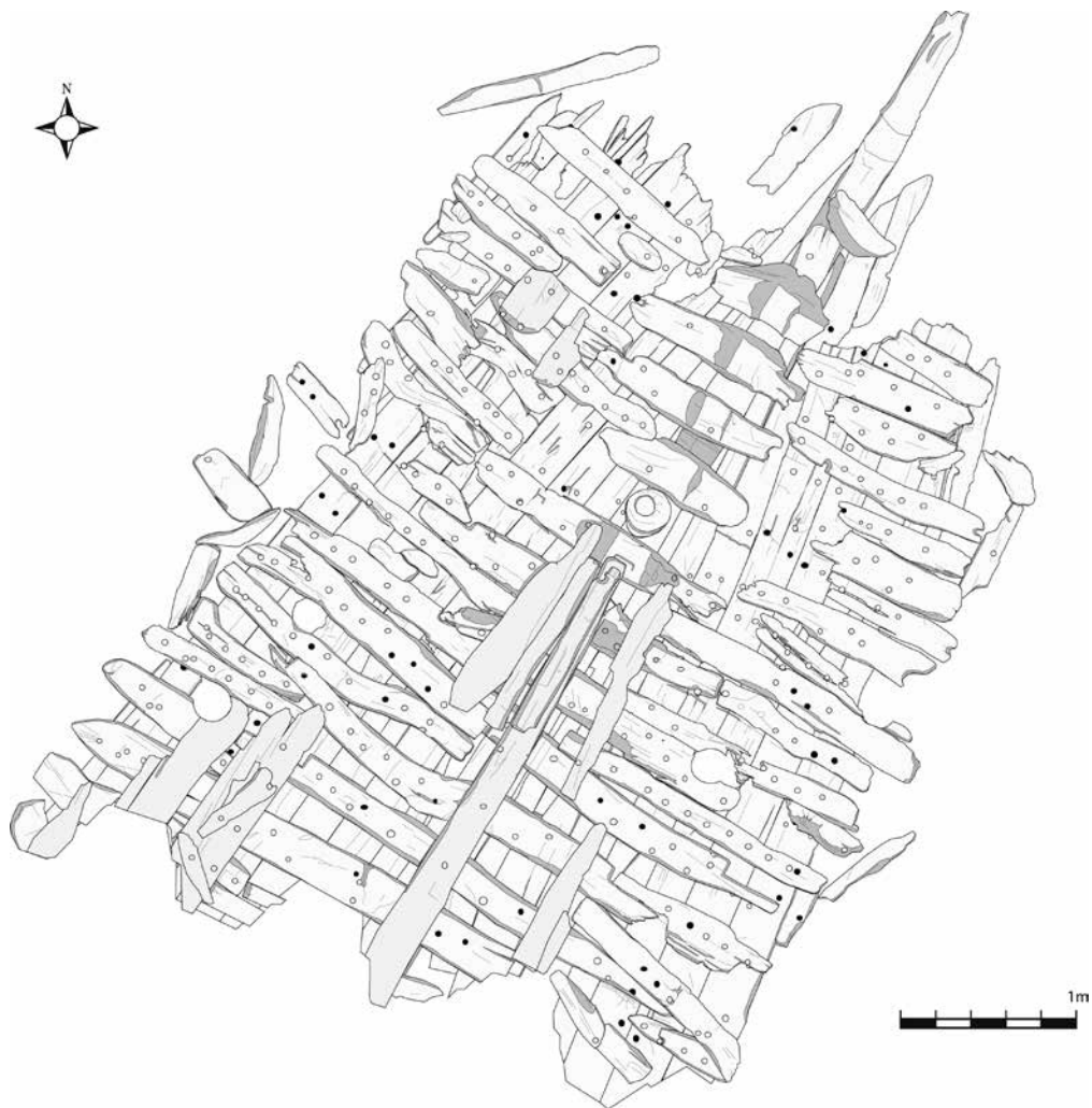
Fig. 2 The boat parts that did survive included a keel, a stern post with stern knee, a keelson, frames, strakes, graving pieces, ceiling planks as well as the foot of a bilge pump (photo: Norwegian Maritime Museum).
