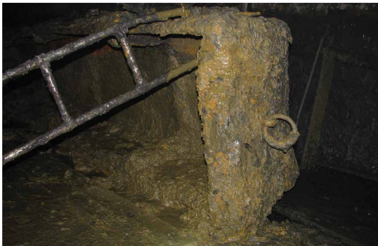
Fig. 2 One of the boats covered with mud found in the adit (photo: courtesy of Coal Mining Museum in Zabrze)
