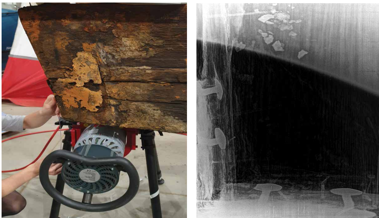
Figs 7a and 7b Radiography as a tool to assess state of preservation of metal parts before the dismantling (photo: B. Galus)
