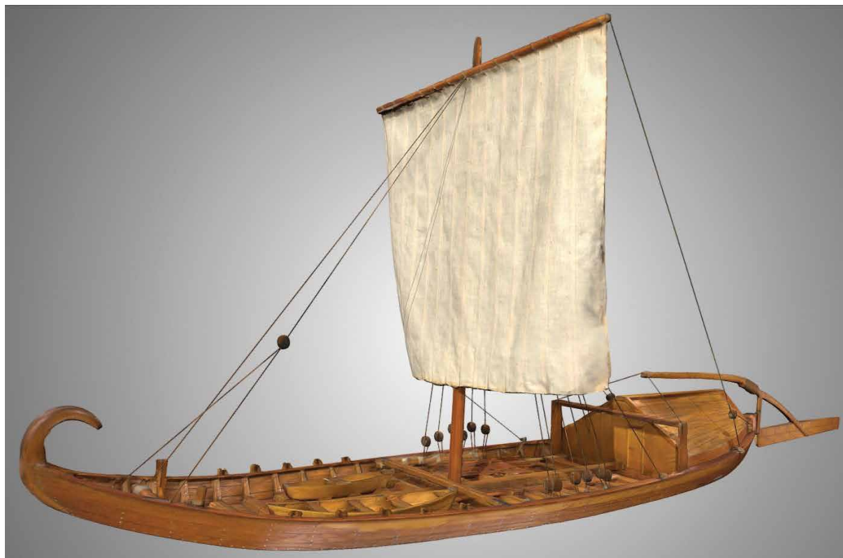
Fig. 8 3D model of a flat-bottomed Vistula vessel (model: T. Bednarz, K. Treder)
