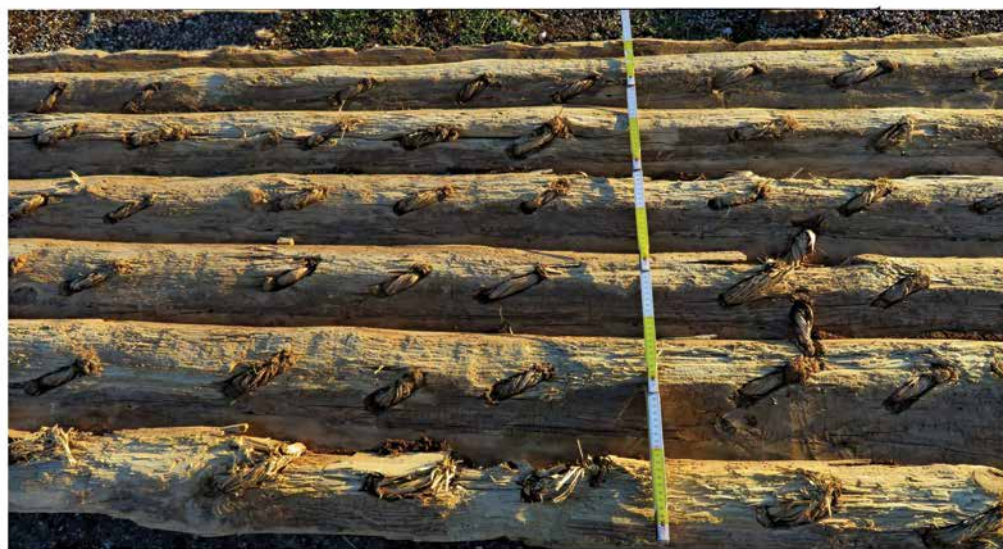
Fig. 6 The sewing and caulking technique of the boards planking of the vessel: 1) the system of connecting and sealing the seams of the board planking; 2) photo of a fragment of the ship's side (drawing and photo: P. Sorokin)
