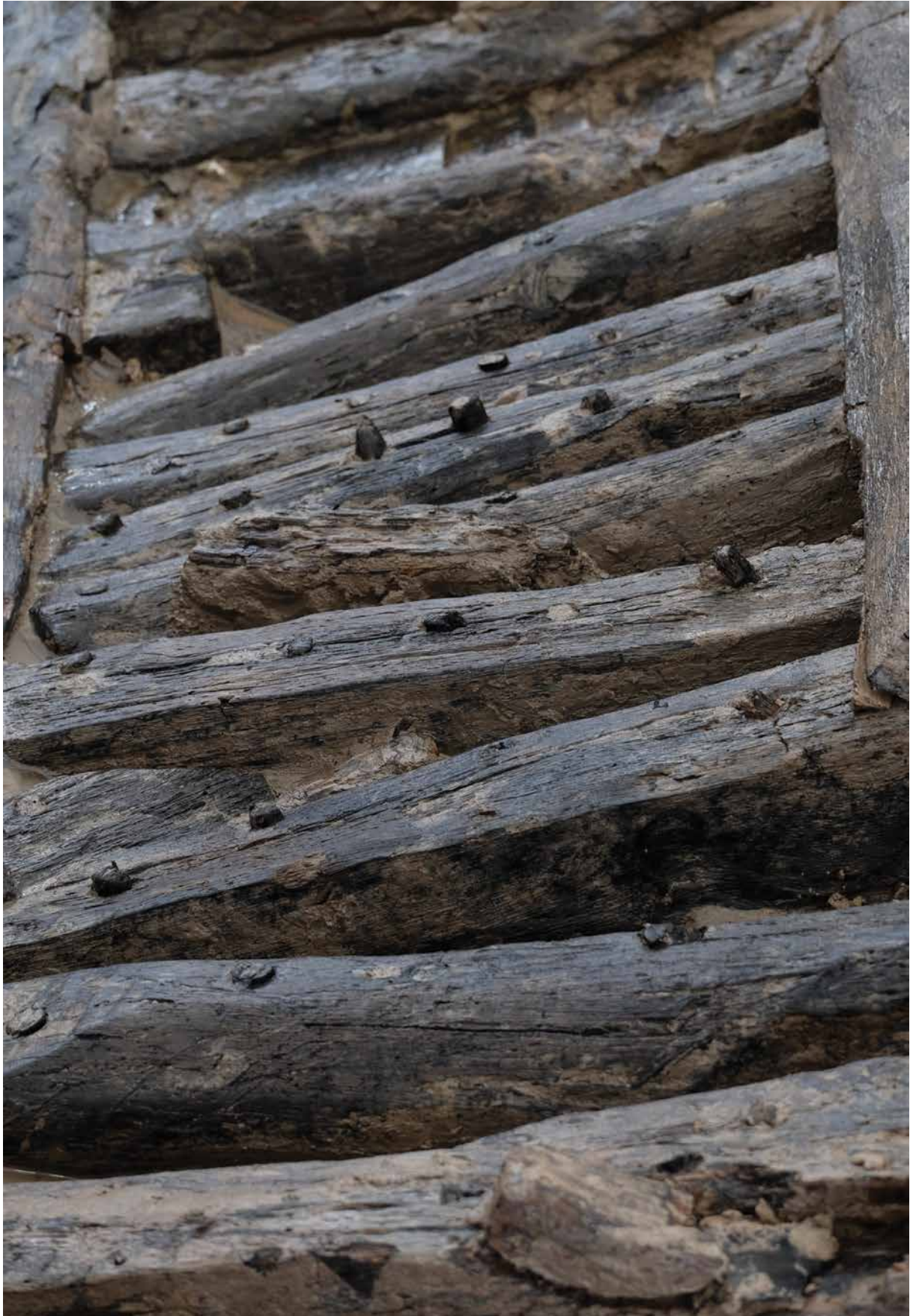
Fig. 6 Detail of the treenails in the starboard frame (photo: P. Ernaux, Inrap)
