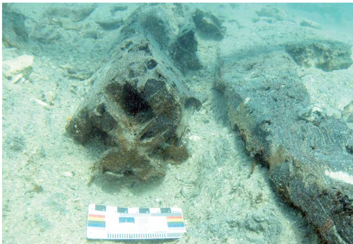
Fig. 5 Keel scarf of Potkamenica shipwreck (photo: M. Kaleb)
