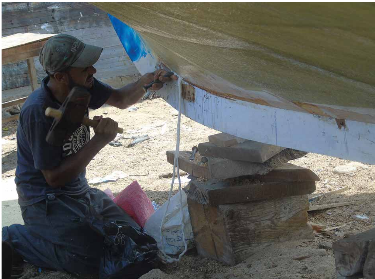
Fig. 6 Caulking a yacht by a labourer who specialized in caulking in Alexandria (photo: A. M. Helmy)
