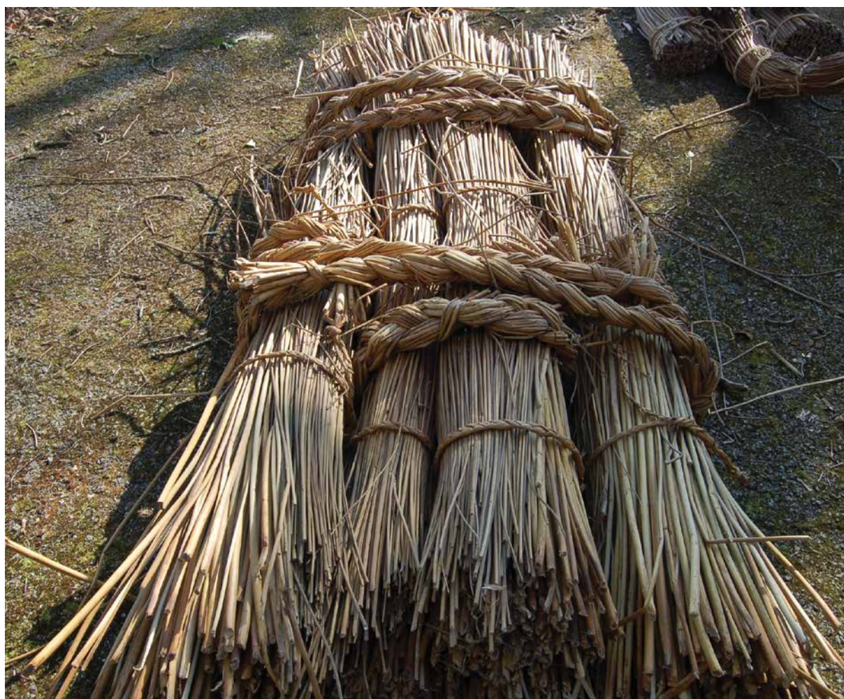
Fig. 5 A simple bundle raft, of no more than 1.5 m 2 , without any framework. This is the most common type of bundle raft cited in the National Folklore Collections. Built by Robert Henshall (photo: D. Tully).
