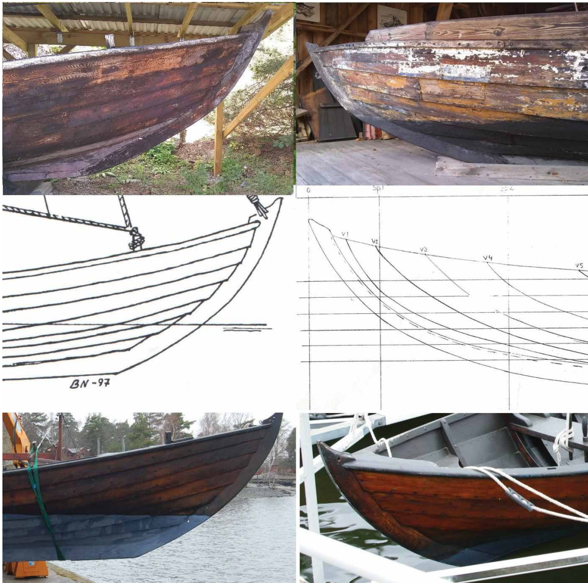
Fig. 4 Stem shape of original boats interpreted with the characteristic shape smoothed out by the replica builders (photo: F. Leijonhufvud).
