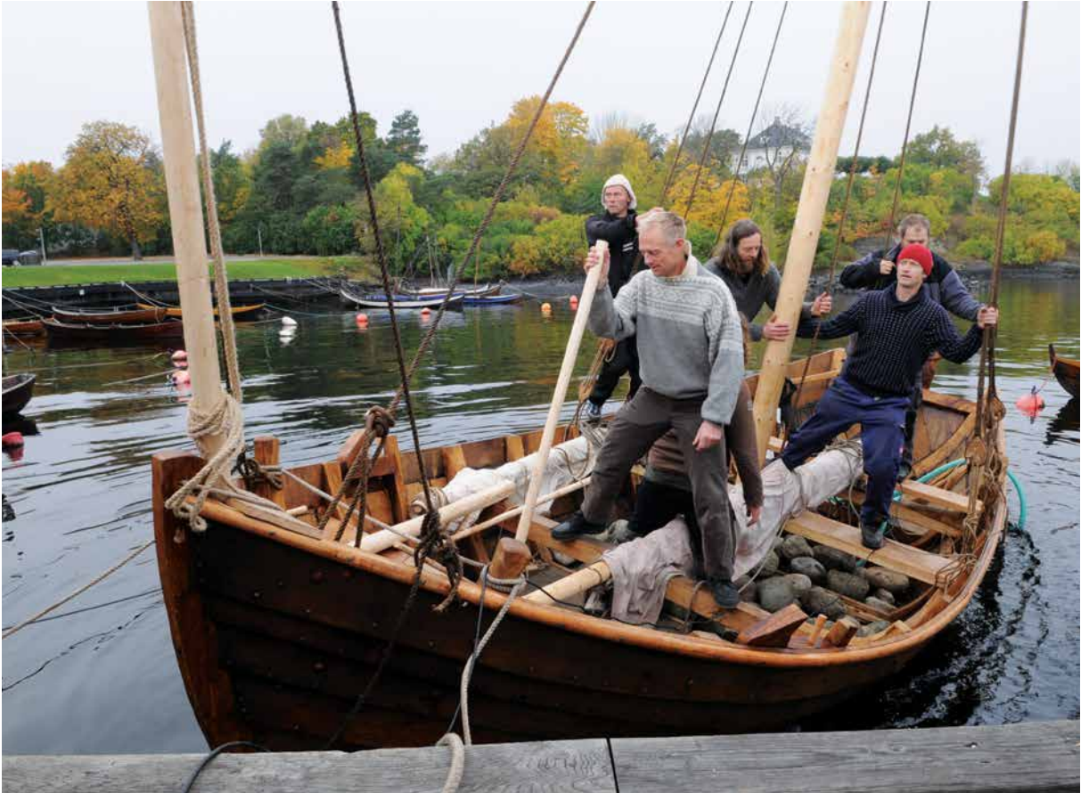
Fig. 6 The small cargo vessel, Vaaghals, has been rigged with one main square sail and one smaller sail in the fore. In the photo, the stability is tested by human force for the first time (photo: K. Steen/NMM).
