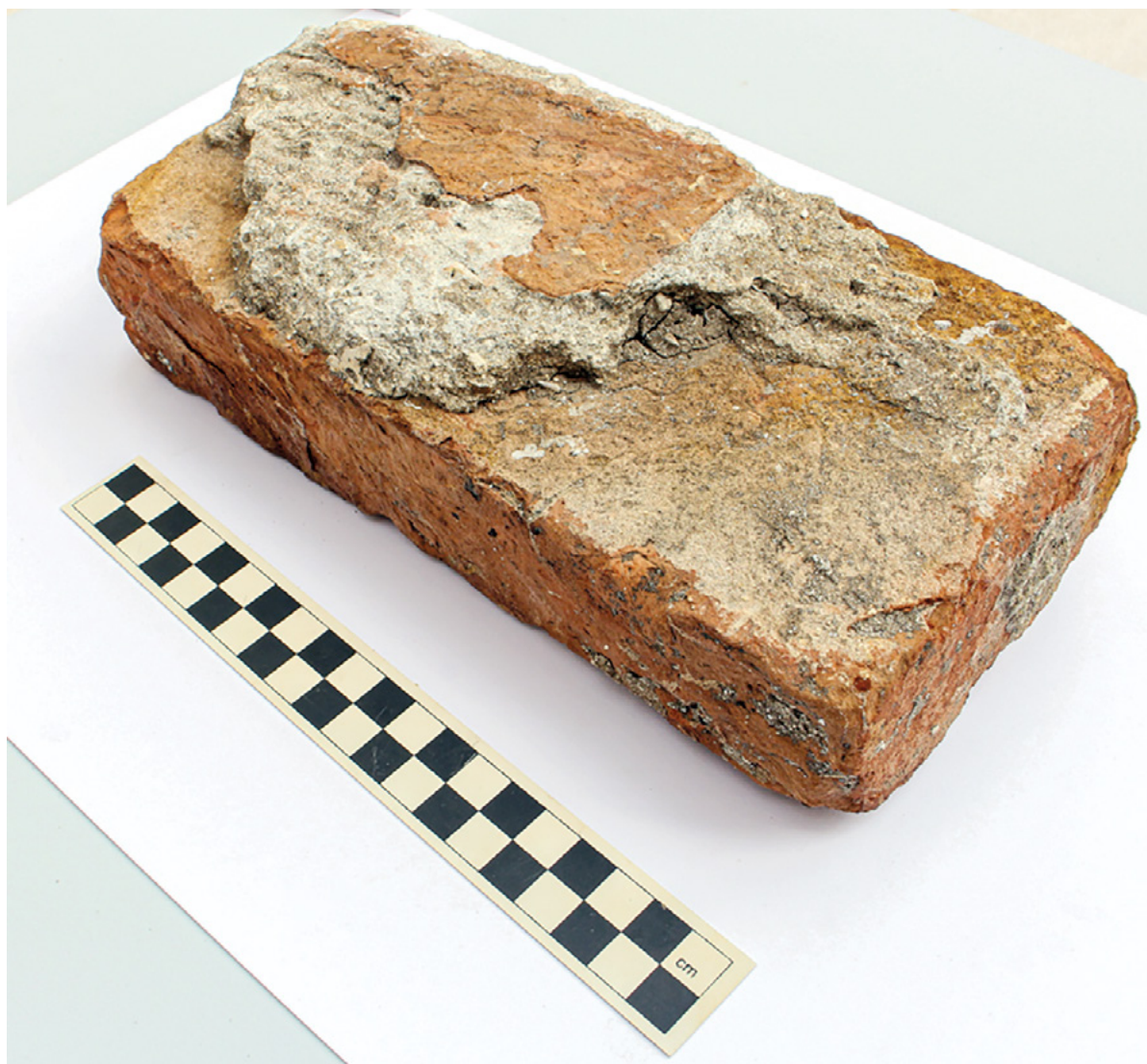
SLIKA 10. Opeka s ostatkom žbuke (snimio: R. Surić) FIGURE 10 Brick with mortar adhering (photo by R. Surić)
