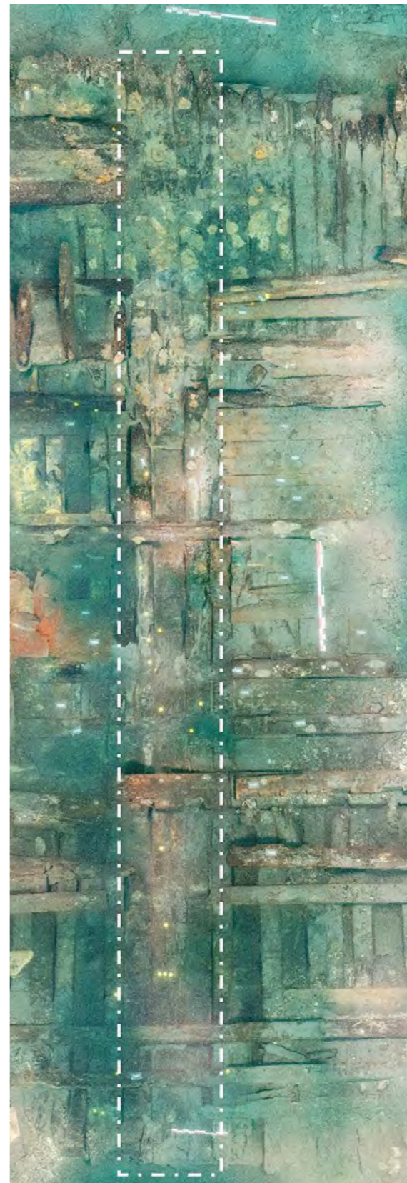
Ortogonalni prikaz modela središnjeg dijela broda s označenim položajem rebrenice i rebrenih nastavaka koji čine glavno brodsko rebro, nakon uklanjanja dijelova temeljnice jarbola i proveza (autor: A. van Zijverden) Orthogonal view of the model of the central part of the ship with the marked position of the floor timber and futtocks that constitute the main frame of the ship, after removing parts of the mast step and stringers (author: A. van Zijverden)
