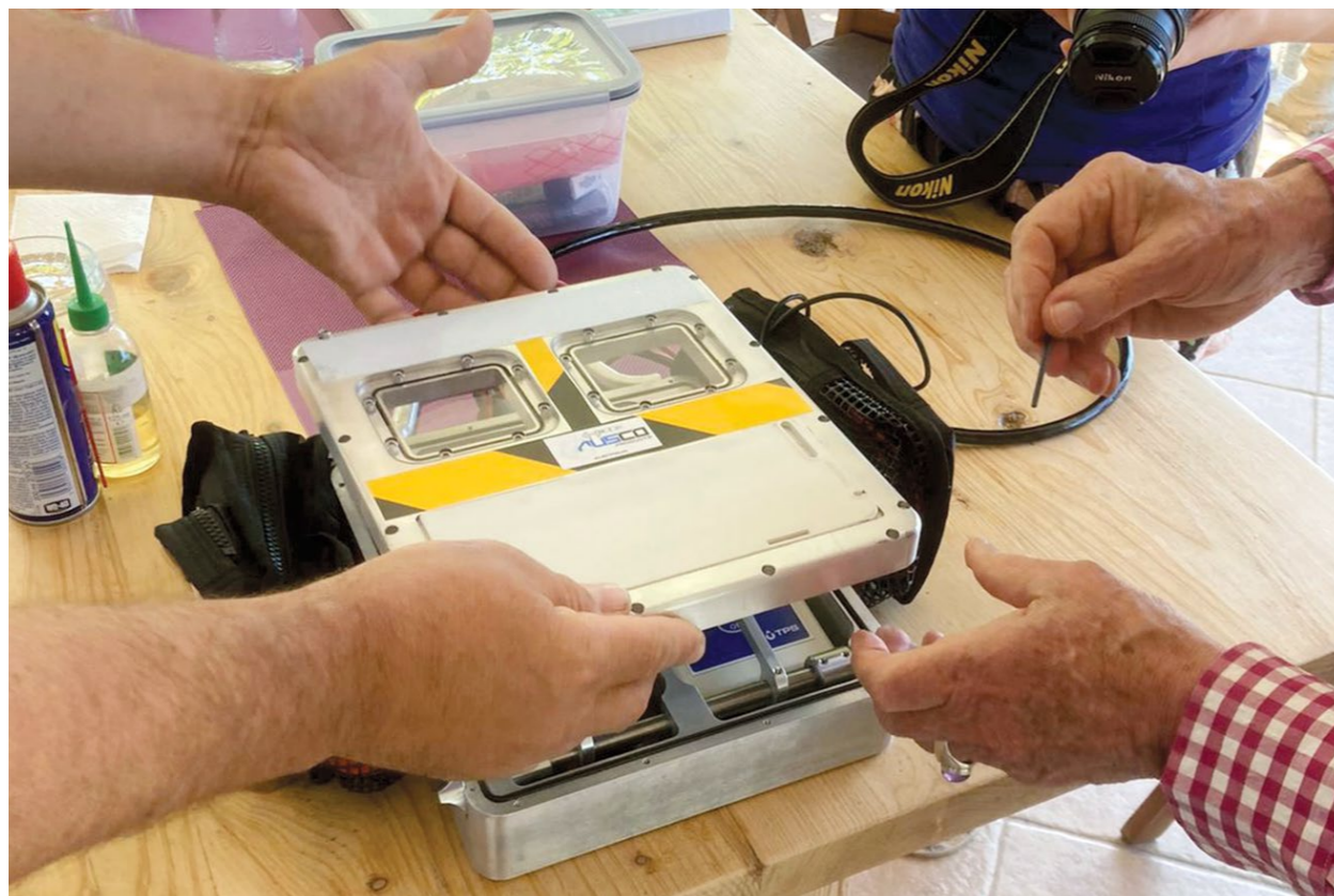
Preprava pH-metra i multimetra u podvodnom kućištu. Uređaju je dodijeljeno ime Duncan (foto: T. Davidowitz) Preparation of a pH-meter and a multimeter in an underwater housing. The device is assigned the name Duncan (photo: T. Davidowitz)
